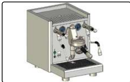
Fig. 9 Portafilter installed, handle pointing to the front
